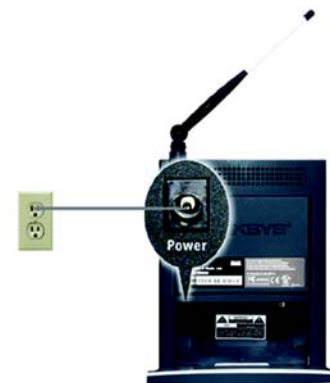
Figure 3-2: Connect the Media Link's Power
